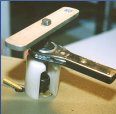
5. Use "T" handle and cut down ratchet wrench to pull nose.
