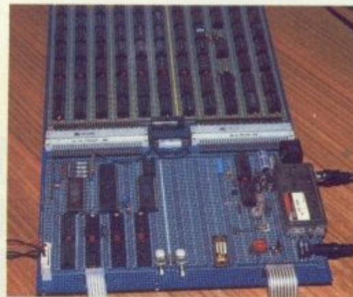
The SAM prototype. The nearer board is the computer itself, while the more cluttered one in the background handles the video logic: this'll be replaced by a single custom chip in the finished machine.
