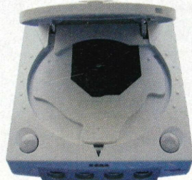
[5] Opening up the CD lid reveals a shallow, solidly built mechanism - there's no exposed catch to detect the drawer closing, but the unit won't activate with the drawer open. No PlayStation disc swapping tricks here!
