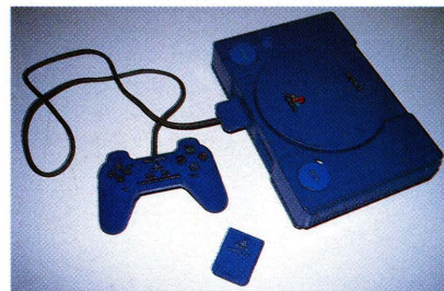
Sony's development hardware began with a series of large target boxes (MW.3, top) and progressed to the twin ISA card system (centre) now in use. Final debugging is done on Sony's blue PlayStations (above)
