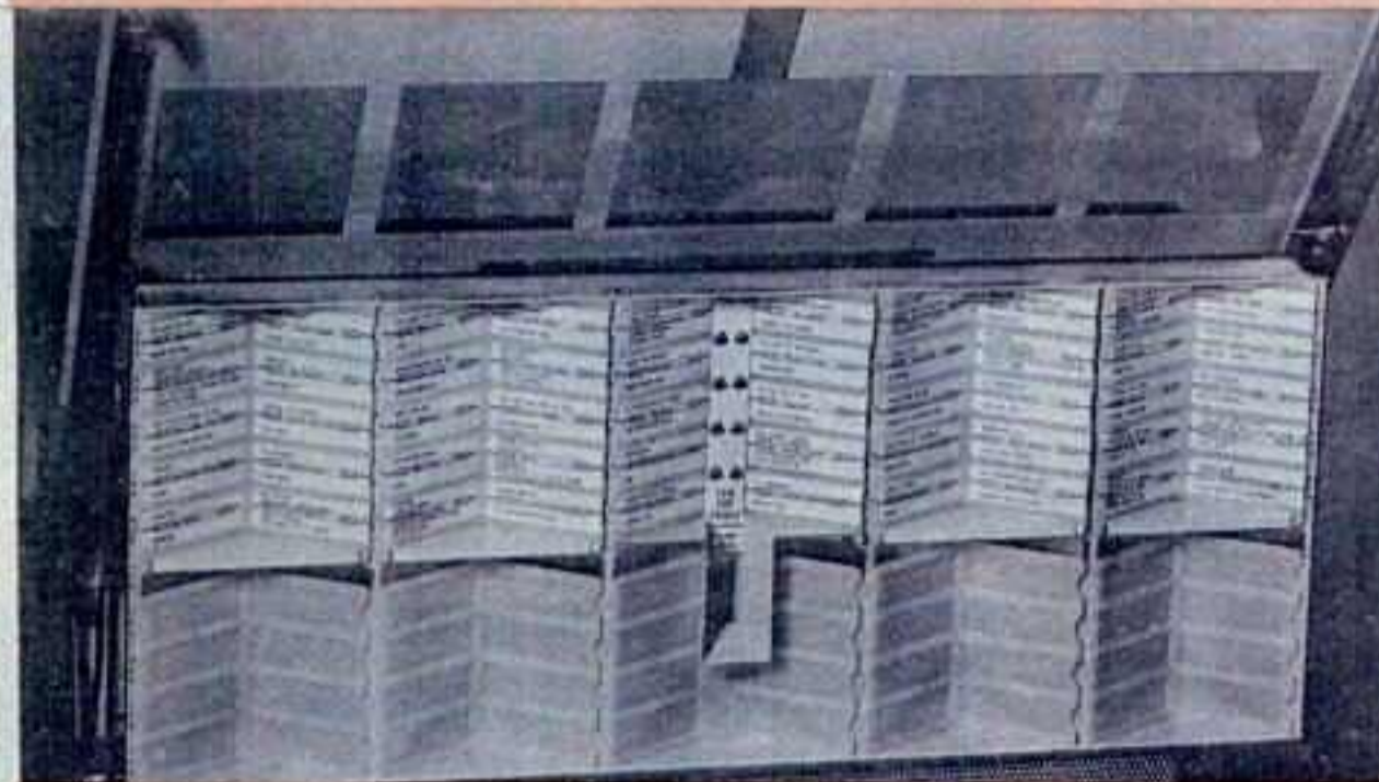
HIGH-SPEED TITLE STRIP CHANGING Entire program unit drops down in vertical position inside raised dome. A terrific time-saver in changing title strips.
