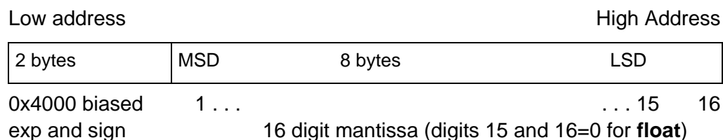
Figure 2.2: Internal TI BCD Floating-Point Representation
