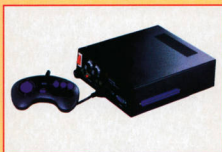
The Super Gun connects to an arcade board for play at home.
