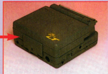
When not in use, the PC Engine LT folds together into a compact package.
