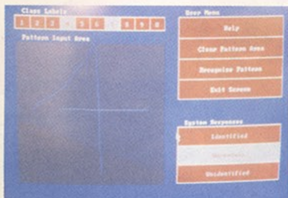
● The numeral recognition system can recognise all the numbers in anyone's handwriting, even say when it is uncertain (for a scrawled figure halfway in between a 4 and a 1, for example) and also say when it can't recognise anything (for a squiggle). A genuine neural network – on a PC!
