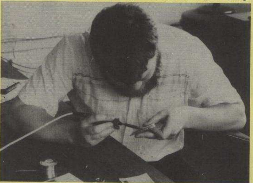
Ian Oliver wrestles with soldering iron and edge connector, to fix a Kempston/128 bug
