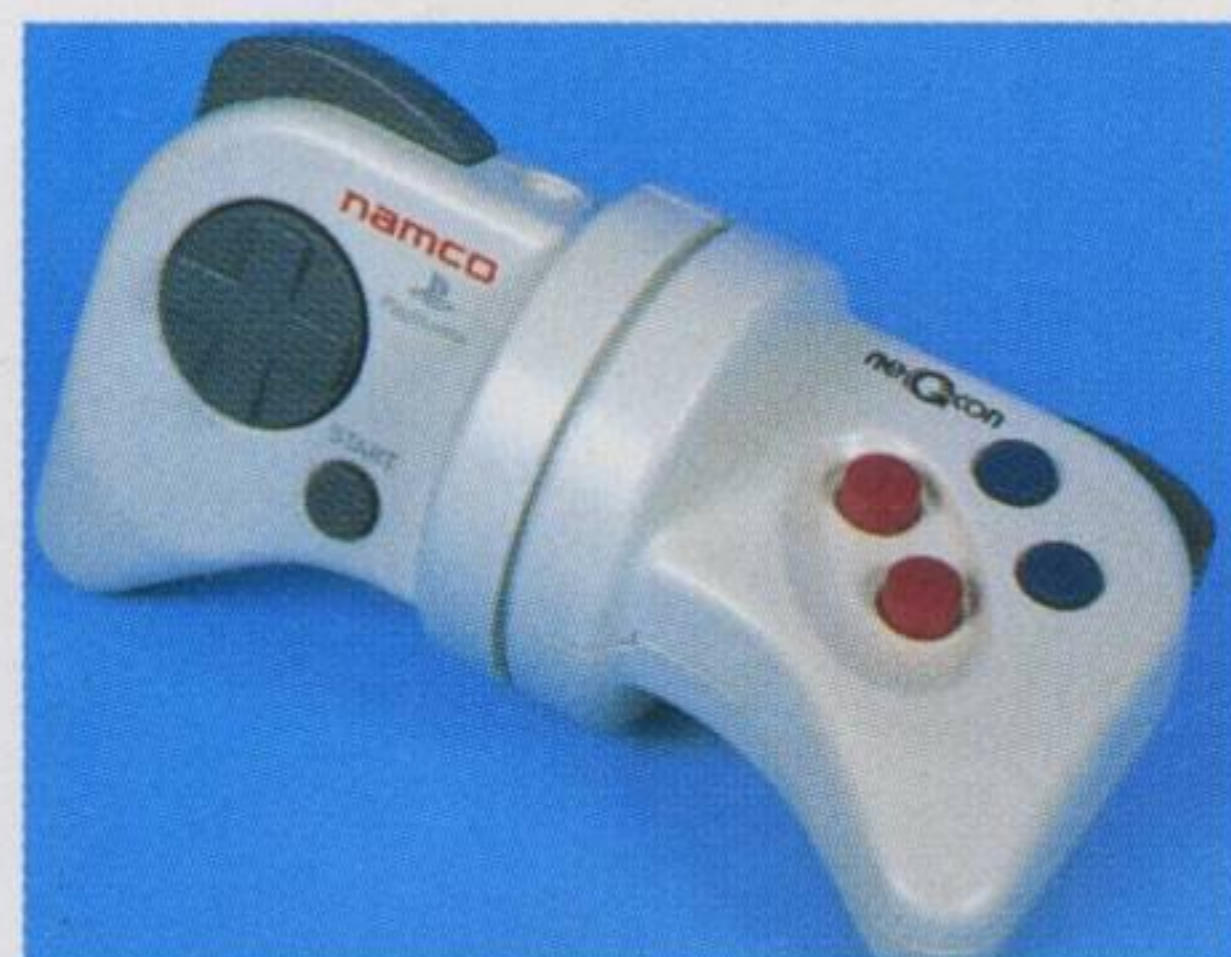
The Negcon for the PlayStation provides analogue control (see letter from Jay Saka)
