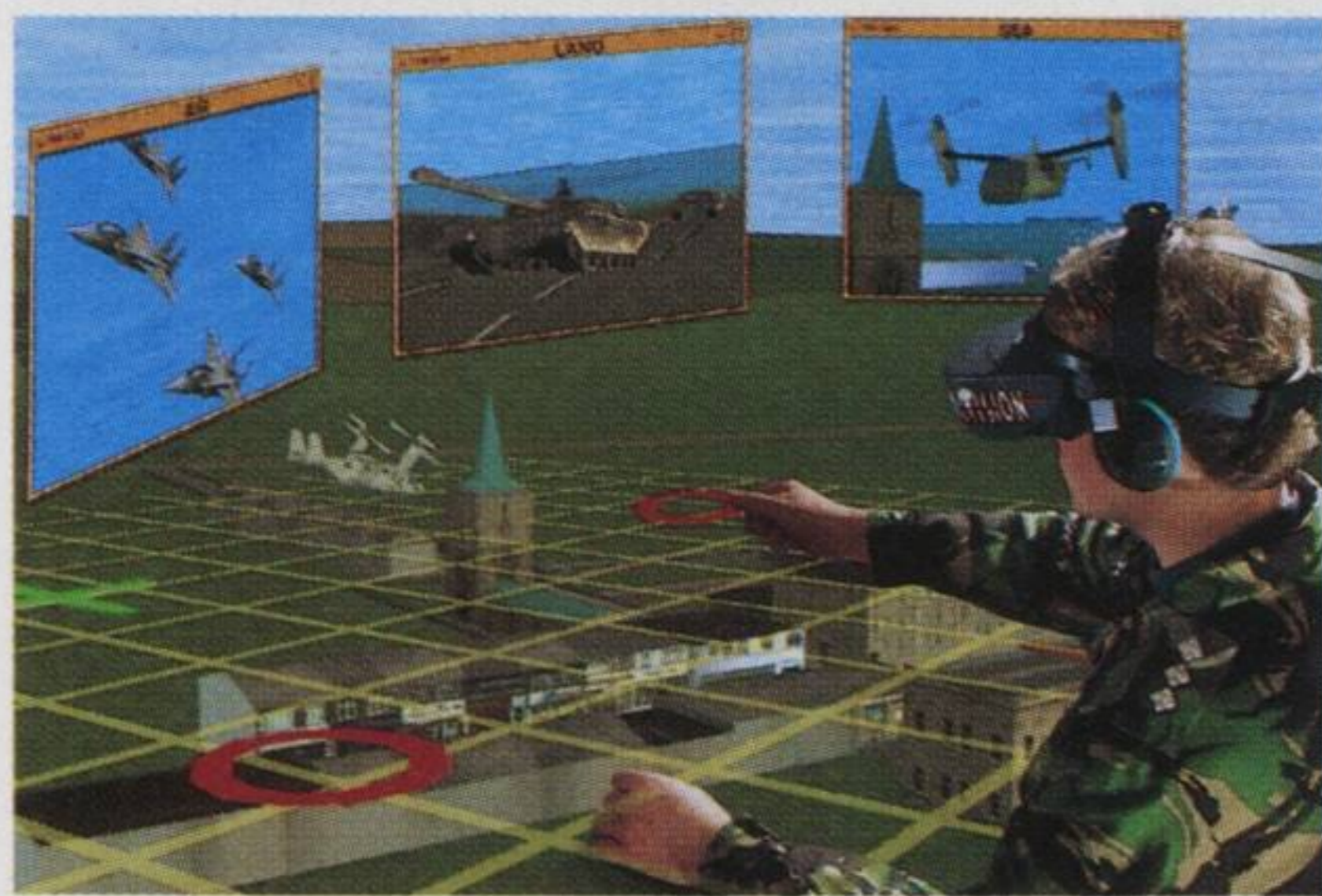
These images from military simulators are generated in realtime. Custom equipment can be combined with the helmets to provide physical training – one sim has pedals that stiffen when the combatant is running uphill
