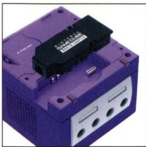
GameCube's expansion port accepts either a Nintendo 56K modem or a broadband unit
