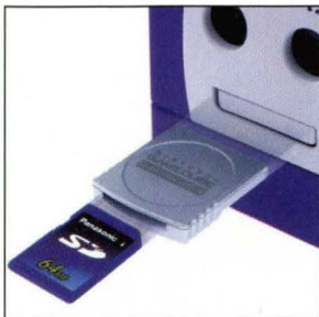
The SD-Digicard adaptor will allow GameCube to be linked up to devices such as digital cameras and mobile phones
