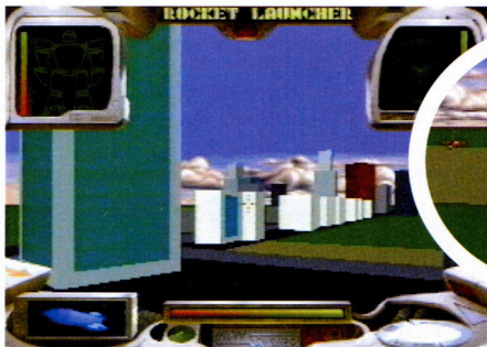
These buildings (above) each consist of 20 polygons. They look very bare at this range because, to keep the frame rate up, the detailing on objects is turned off when you move beyond a certain distance
