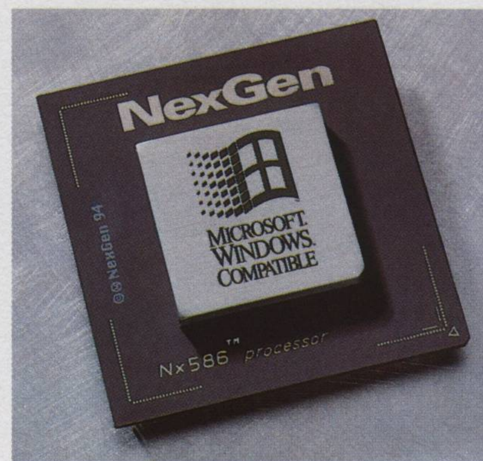
The NextGen Nx586 is one of the first of a new breed of RISC-based processors which can run Intel 80x86 code
