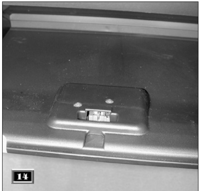
The glove box lock assembly is held in with 2 screws that must be removed.
