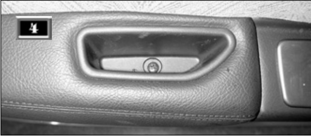
Inside the door pull cavity is another panel screw that must be removed.
