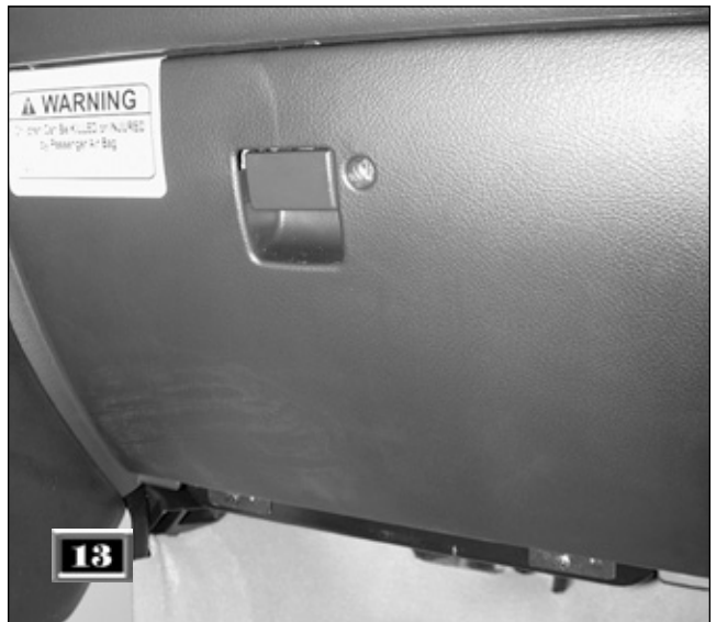
The glove box lock cylinder is part of the glove box handle latch assembly also.
