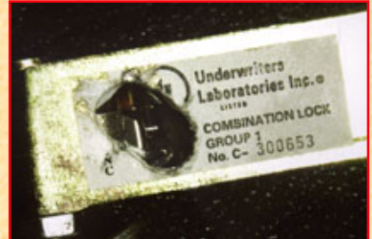
4. Holes(s) through the side of the lock case showing the pin and bolt. The pin is easy to see once you have drilled this hole.
