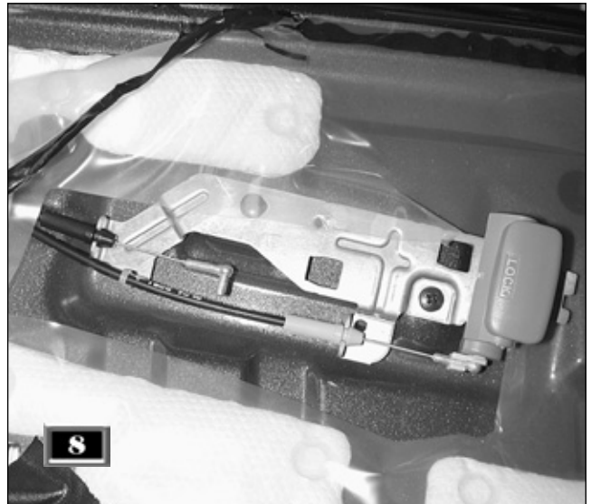
Here's a look at the cable linkage for the inside door release and the inside door lock button.
