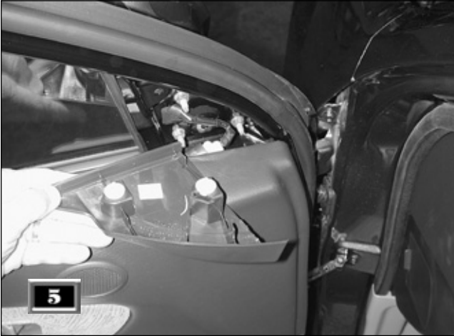
On the very top forward section of the panel is a small triangular plastic trim panel that unsnaps and must be removed.
