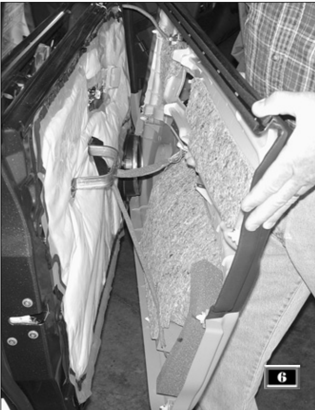
The common push-in plastic clips now only hold on the panel. Start at the bottom of the panel and work your way up as gently but firmly pull the panel away from the structure of the door.
