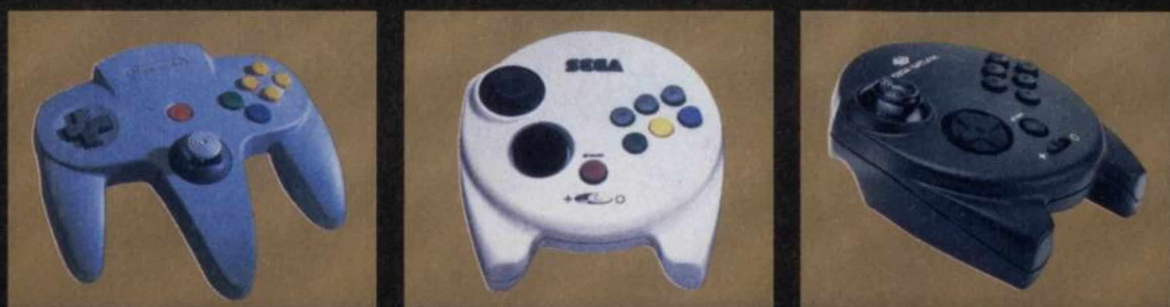
An analogue stick takes centre stage on the Nintendo 64's controller (left); Sega's reply for the Saturn (Japanese version, centre, western version, right) uses a more pad-like analogue device
