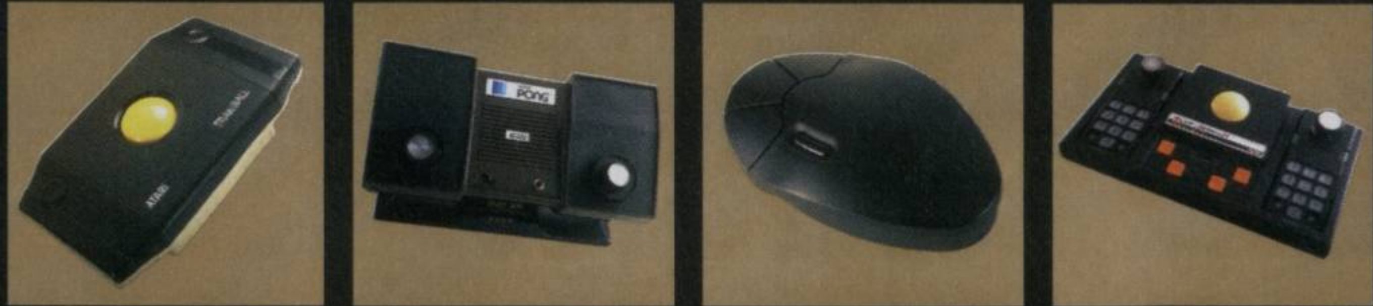
From left to right: Atari's trackball device, the precursor to the mouse, was used to control crosshair sights in Missile Command ; Super Pong , Atari's home version of its ground-breaking coin-op, was an early exponent of analogue 'paddle' controllers; Sega's mouse device for the Saturn; a Colecovision-compatible trackball
