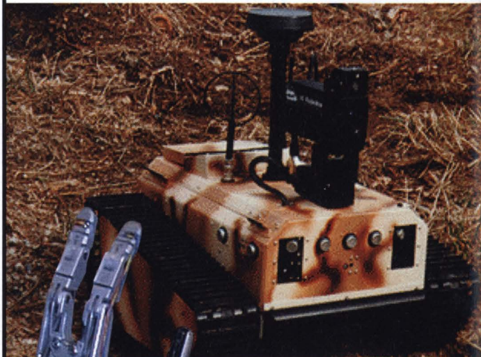
The ROAMS recon-robot sneaks behind enemy lines using satellite guidance and a remotely-controlled video camera to avoid things like traps. And stairs.
