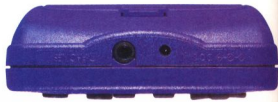
Ⓒ The top of the new unit, the on/off switch has been replaced by the cool infrared port.
