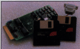
The key to Color Dreams' development system is a circuit board that connects an IBM PC to the NES's cartridge slot.
